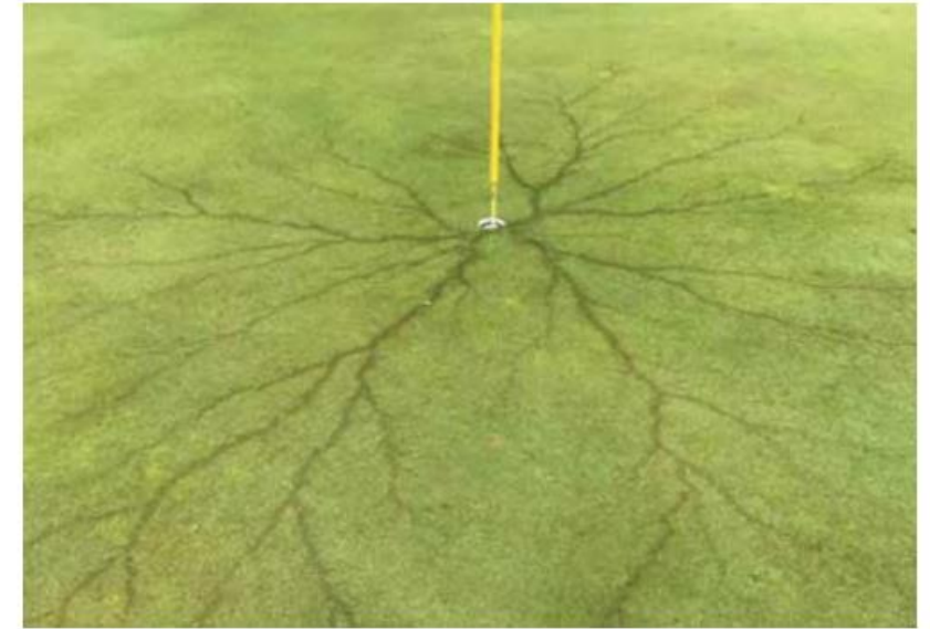
Fig. 1. Soil breakdown near the current admitting point of a grounding system.
