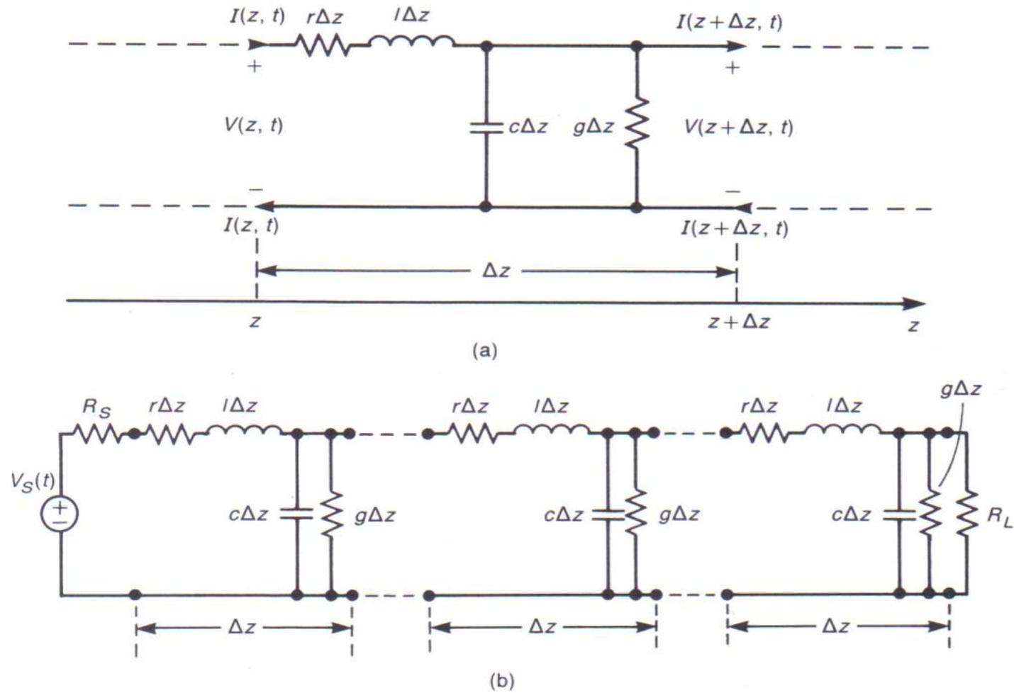
**FIGURE 4.3** The per-unit-length equivalent circuit of a two-conductor line for the TEM mode of propagation: (a) the equivalent circuit for a  $\Delta z$  section; (b) modeling the entire line as a cascade of  $\Delta z$  sections from which the transmission line equations are derived in the limit as  $\Delta z \rightarrow 0$ .
