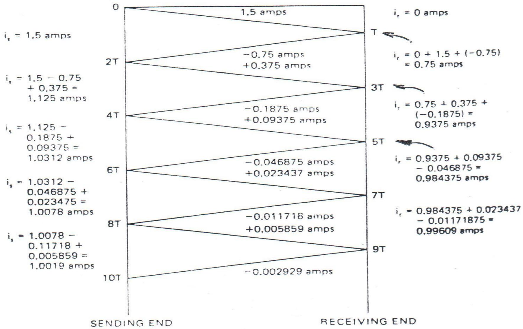
Figure 8-10. Current Bounce Diagram.
