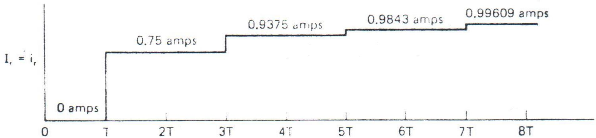
Figure 8-11.  $I_s$  and  $I_r$  as functions of time.
