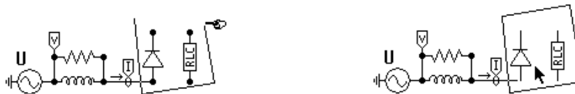
Fig. 3.15 - Drawing a polygon: First double click on white space, click the left mouse button at each corner of the polygon, then click the right button to enclose the polygon.
