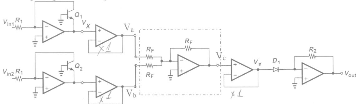
a)  $\frac{V_{in1}}{R_1} \rightarrow V_x$        $I_{C1} = I_{SQ1} \cdot \exp\left(\frac{V_{BE}}{V_T}\right)$        $I_{R1} = I_{C1}$        $\frac{V_{in1}}{R_1} = I_{SQ1} \exp\left(-\frac{V_x}{V_T}\right) \Rightarrow \exp\left(-\frac{V_x}{V_T}\right) = \frac{V_{in1}}{R_1 \cdot I_{SQ1}}$
