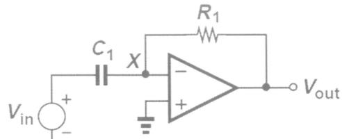
•  $\frac{V_i}{Z_1} - \frac{V_x}{Z_2} = \frac{V_x - V_o}{R_1} \Rightarrow \frac{V_i}{Z_1} = \frac{V_x - V_o}{Z_2} \Rightarrow V_o = -Z_2 \frac{V_i}{Z_1}$
