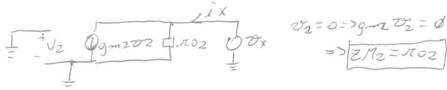
$$v_2 = 0 \Rightarrow g_{m2} v_2 = 0 \Rightarrow Z_{M2} = r_{02}$$
