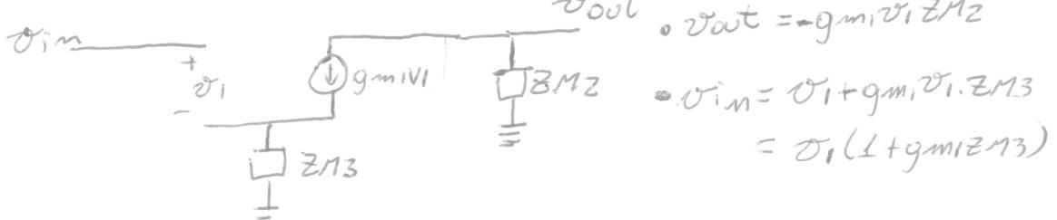
$$v_{out} = -g_{m1} v_1 Z_{M2}$$
