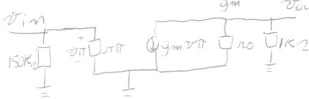
$$r_{out} = \frac{V_{out}}{\omega_{pi}} = r_o // 1k\Omega \approx 994,3632\Omega$$
