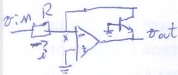
$$v_{out} = -V_T \ln \frac{v_{in}}{R I_S}$$
