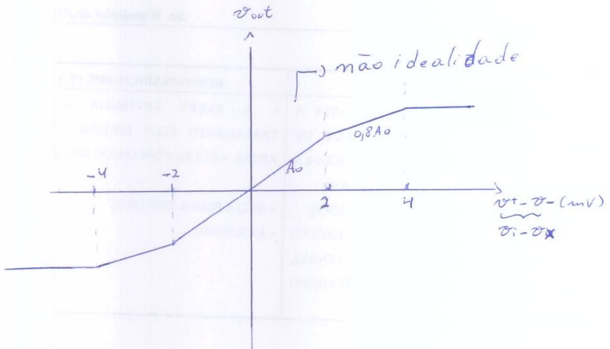
•  $(v_i - v_x) = 2\text{mV} \Rightarrow v_i = \left(1 + \frac{A_0}{5}\right) \cdot 2\text{mV}$
