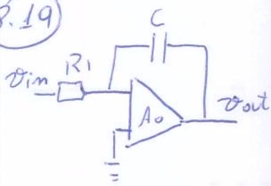
$$A_0 = \frac{v_{out}}{v_{in}} = \frac{-1}{sC R_1} \Rightarrow A_0 = \frac{-1}{R_1 C s}$$
