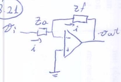
$$v_{out} = (v_+ - v_-) \cdot A_0 \Rightarrow v_{out} = -A_0 v_-$$
