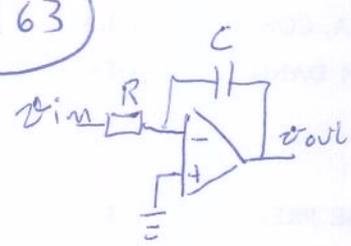
$|v_{out}(t)| = \alpha t = \left| -\frac{1}{RC} \right| t = \frac{10V}{\mu s} t$
