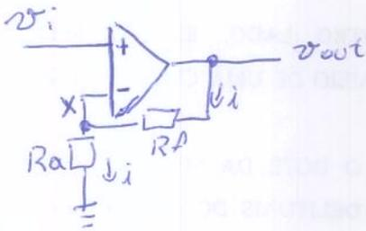
$$i = \frac{v_x}{R_a} = \frac{v_{out}}{R_f + R_a} \Rightarrow v_x = \frac{R_a v_{out}}{R_f + R_a}$$
