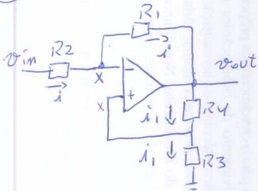
$$\begin{cases} i = \frac{v_{in} - v_x}{R_2} = \frac{v_x - v_{out}}{R_1} \\ i_1 = \frac{v_x}{R_3} \\ v_{out} = (R_3 + R_4) \cdot i \Rightarrow v_{out} = \frac{R_3 + R_4}{R_3} \cdot v_x \end{cases}$$
