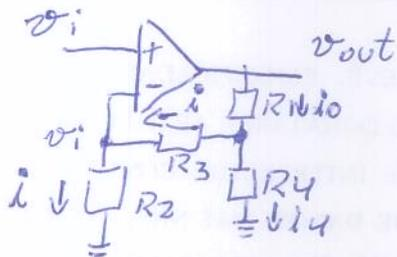
$$i_0 = \frac{v_{out} - v_{R4}}{R_1} = \frac{v_{out} - (v_i + v_{R3})}{R_1}$$
