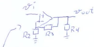
•  $R_1 \rightarrow \infty \Rightarrow \frac{v_{out}}{v_{in}} = \frac{R_3 + R_2}{R_2} \Rightarrow \frac{v_{out}}{v_{in}} = 1 + \frac{R_3}{R_2} \Rightarrow$  OK, ganho do amp. n̄ inv. ( $R_f = R_3, R_a = R_2$ )
