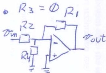
$$\frac{v_{out}}{v_i} = -\frac{R_1}{R_2} \Rightarrow OK$$
