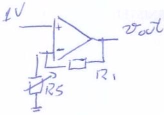
$$v_{out} = v_{in} \cdot \left(1 + \frac{R_1}{R_S}\right)$$
