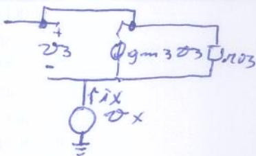
$R_{M3} = r_{o3} \parallel \frac{1}{g_{m3}}$
