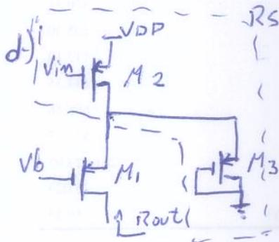
obs: ver obs 7.33-c  $\Rightarrow R_S = R_{M2} \parallel R_{M3}$
