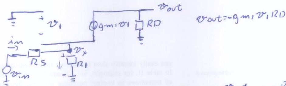
$$v_{out} = -g_{m2} v_x R_D$$
