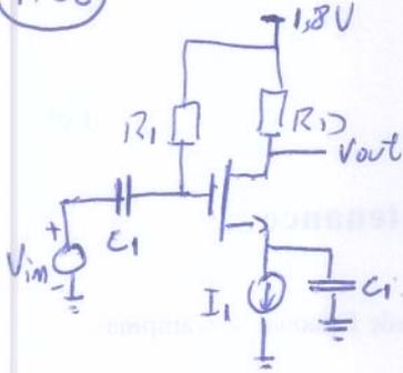
$I_D = I_1 = 1 \text{ mA}$       $\lambda = 0$       $V_{TH} = 0.4 \text{ V}$
