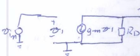
$v_{out} \Rightarrow A_v = \frac{v_{out}}{v_{in}} = -g_m R_D$
