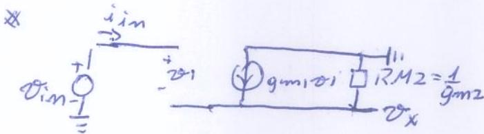
$$v_x = g_{m1} v_1 \cdot \frac{1}{g_{m2}}$$
