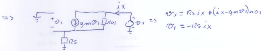
$$v_x = R_S i_x + (i_x - g_m v_1) r_{o1}$$
