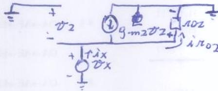
$$v_x = -v_2 \Rightarrow v_x = -v_2 = v_{r_{o2}}$$
