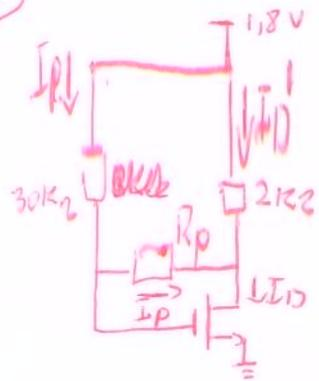
$R_p \rightarrow \infty \Rightarrow V_{GS} = V_{DS} + 100\text{mV} \rightarrow \text{SAT}$
