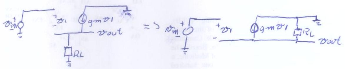
$v_{out} = g_m v_1 R_L$
