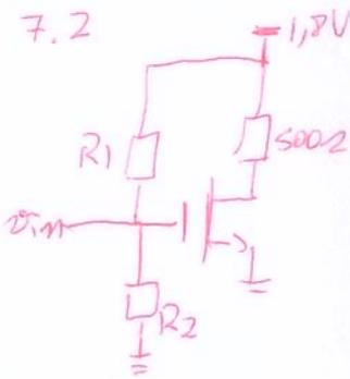
$$\begin{aligned} \frac{W}{L} &= \frac{20}{0,18} \\ R_{in} &= 20 \text{ k}\Omega \\ I_D &= 1 \text{ mA} \\ \lambda &= 0 \\ V_{TH} &= 0,4 \text{ V} \\ \mu_n C_{ox} &= 200 \cdot 10^{-6} \text{ A} \end{aligned}$$
