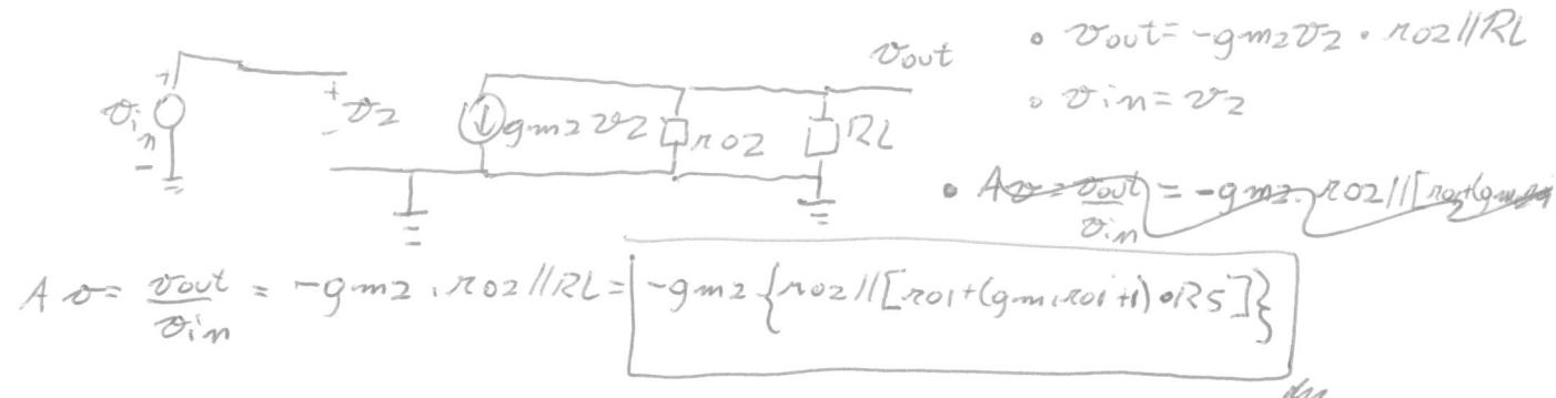
$$\bullet v_{out} = -g_m v_2 \cdot r_{102} / RL$$
