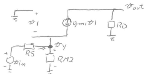
$$\frac{\partial v_{out}}{\partial v_{in}} = -g_m 1 R_D$$
