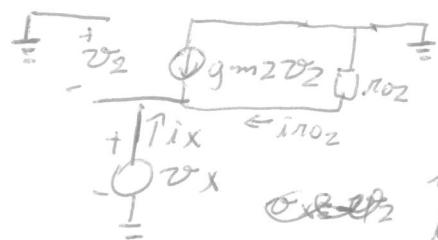
$$v_x = -v_{22} \quad i_x = g_{m2}v_{22} + i_{r_{o2}}$$
