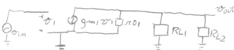
$$\frac{v_{out}}{v_{im}} = A_v = -g_{m1} \cdot \left( r_{o1} \parallel r_{o2} \parallel r_{o3} \parallel \frac{1}{g_{m3}} \right)$$
