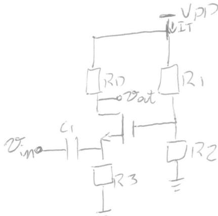
$$\begin{aligned}V_{DD} &= 1,8 \text{ V} \\P &= 2 \text{ mW} \\A_\Omega &= 50 \\R_3 &= 500 \Omega \\Q &= 500 \text{ A} \\g_m &= 136,4 \text{ S} \\I_{in,ox} &= 100 \mu\text{A}/\sqrt{\text{V}^2} \\V_{TH} &= 0,5 \text{ V} \\&\lambda = 0 \\W &= 244 \text{ } \mu\text{m}\end{aligned}$$
