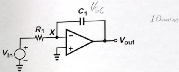
a)  $v_x = 0 \Rightarrow \frac{v_{in}}{R_1} = \frac{0 - v_{out}}{\frac{1}{sC}} \Rightarrow v_{out} = -\frac{1}{sCR} v_i$  ou
