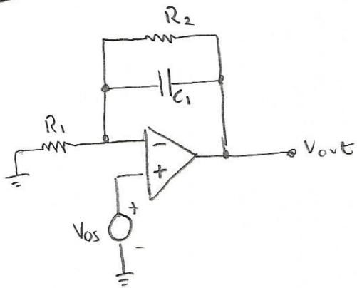
$$V_{out} = V_{os} \left( 1 + \frac{R_2}{R_1} \right)$$
