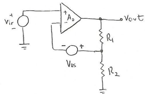
$$V_{IR} + V_{OS} = V_{out} \frac{R_1}{R_1 + R_2}$$
