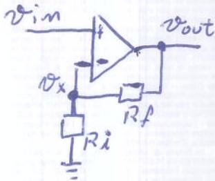
$$\Rightarrow \frac{v_x}{R_i} = \frac{v_{out}}{R_f + R_i} \Rightarrow v_{out} = v_x \left( \frac{R_f + R_i}{R_i} \right)$$
