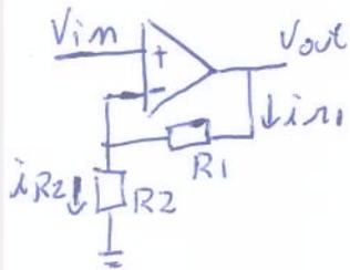
$$A_o \rightarrow \infty \Rightarrow v_+ = v_- = v_{in}$$
