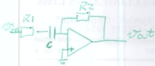
$$\frac{v_{out}}{v_{in}} = \frac{-R_2}{R_1 + \frac{1}{sC}} = \frac{-R_2}{R_1 s C + 1}$$
