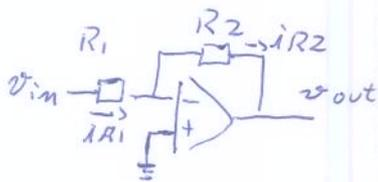
$$\bullet v_- = v_+ = 0 \Rightarrow i_{R1} = i_{R2}$$
