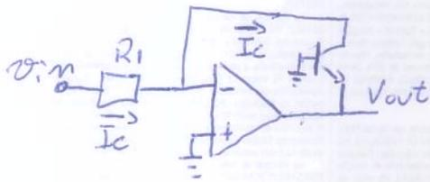
$$\rightarrow I_c = \frac{v_{in}}{R_1}$$
