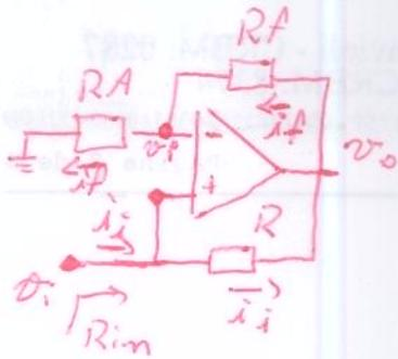
$$i_i' = \frac{v_o - v_i}{R_A} = \frac{v_i}{R_A} \Rightarrow v_i = \frac{R_A(v_o - v_i)}{R_A}$$
