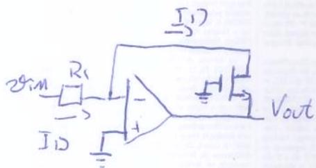
$$\rightarrow I_D = \frac{v_{in}}{R_1}$$
