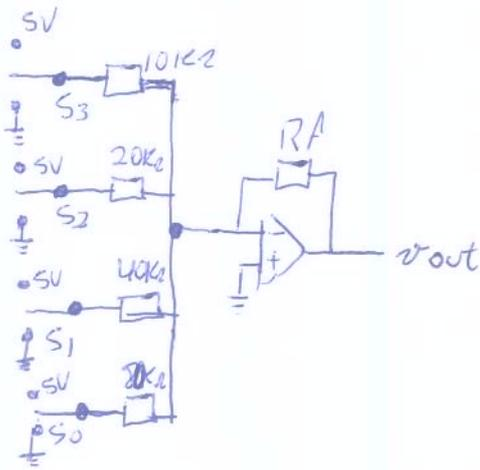
$$v_{out} = \frac{R_f}{80} \cdot v_0 + \frac{R_f}{40} \cdot v_1 + \frac{R_f}{20} \cdot v_2 + \frac{R_f}{10} \cdot v_3$$
