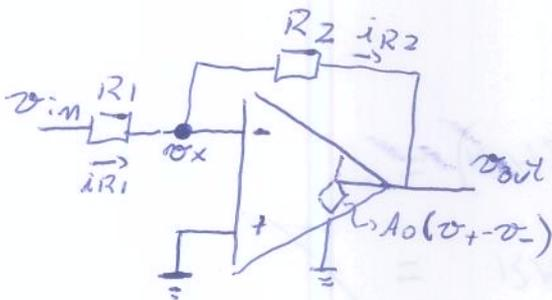
$$\bullet v_{out} = A_o(v_+ - v_-)$$
