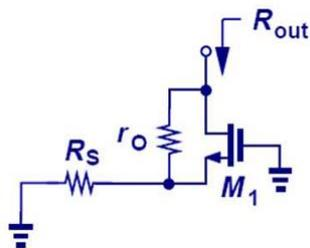
$$R_{out} = (1 + g_m r_o) R_s + r_o$$
