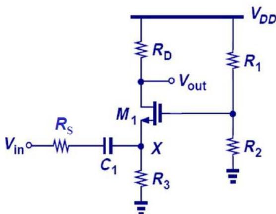
$$\frac{v_{out}}{v_{in}} = \frac{R_3 \parallel (1/g_m)}{R_3 \parallel (1/g_m) + R_S} g_m R_D$$
