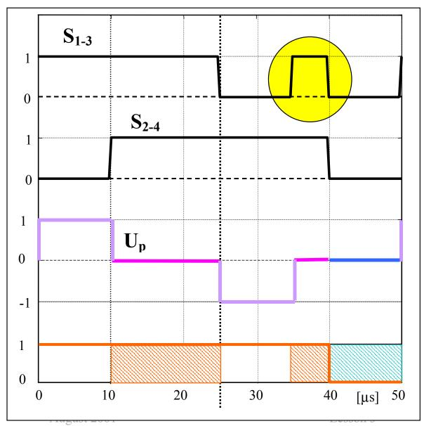
Symmetrical positioning of switching pulses requires two additional commutations
