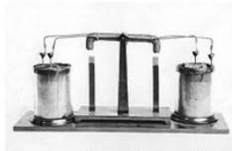
Reconstruction of Henry's original oscillating electromagnet motor. N.M.A.H. Cat. No. 244,904. Smithsonian neg. no. 24,976-A.
